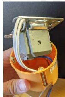
Through clever installation, the SMI interface can be exchanged at any time with a network socket with RJ45 connections or Wifi.
