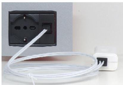
On the SMI interface any type of media converter or switch can be used with the POF SMI patch cable.
